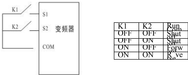
Two-wire operation mode 2 schematic diagram
